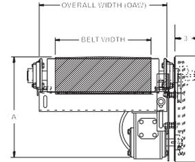
Model 450BOS slider bed belt conveyor is one of the most popular and common means of transporting goods for packing, testing, inspecting and a variety of assembly line operations. 450BOS features a box style slider bed, ideal for workers stationed alongside the conveyor.
